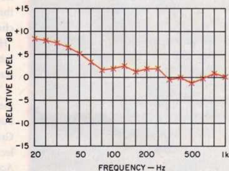
FIG. 5— AUGMENTATION, IN THIRD OCTAVES, FOR A WOOFER SPACED 10, 36, AND 60 INCHES FROM NEAREST ROOM BOUNDARIES; PLOT HAS BEEN REDRAWN FROM BESTPLACE OUTPUT.
